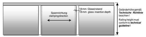
**Note:** If the types of glass and the dimensions listed in Table B are used, only static structural proof calculations are required.
