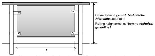
**Note:** If the types of glass and the dimensions listed in Table B are used, only static structural proof calculations are required.
