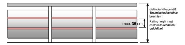
The type of glass used shall be selected from Table A, glazing not intended to protect against falls. The spacing between horizontal bars should not exceed approx. 35 cm.
